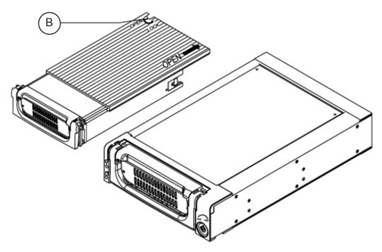
Turn the screw (A) clockwise to open the cover. After HDD is installed, sliding back the cover and turn the screw (A) counter-clockwise to prevent the cover from loosing.
