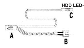
A. Connect to pins on the motherboard (wire white color is "-"),
